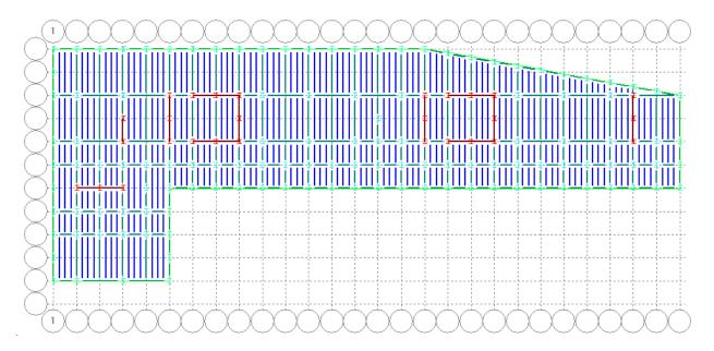
Red indicates braced frame Blue indicates open-web joists Dark green indicates composite beams Light green indicates columns
